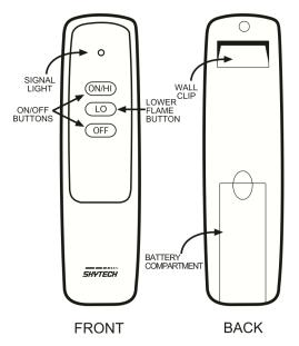
This remote control SYSTEM offers the user a battery-operated remote control to power an ON/OFF latching solenoid such as the one used with the AFLMF valve kit.
